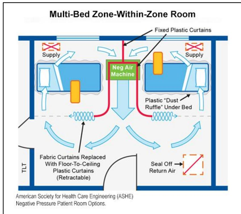
the negative pressure zone into general room air outside the enclosure. Dust ruffles or similar are provided under the bed(s) to minimize air movement below the bed(s). Exhaust air grills are sealed off. Supply air vents may be inside or outside the containment area with openings as appropriate in the plastic sheeting to permit re-entry of clean room air. The door to the patient room
