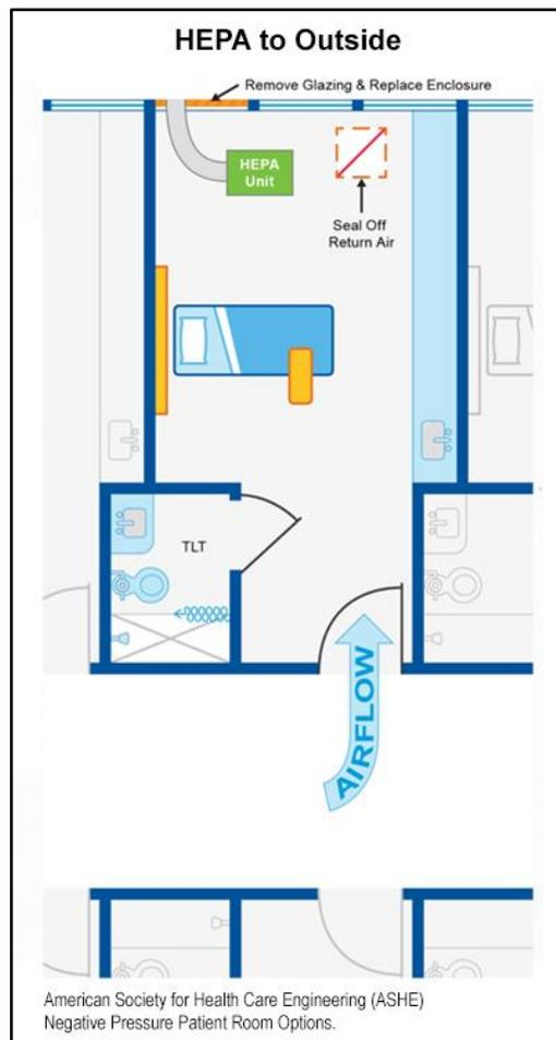
achieve a pressure differential of negative 2.5 Pa with the door closed. The patient room is now under negative pressure relative to the corridor. Pressure should be monitored daily.
