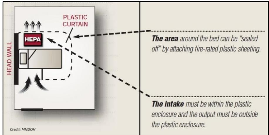
plastic sheeting. A HEPA-filtered negative air machine is strategically placed within the sealed off negative pressure zone. The intake of the negative air machine must be within the plastic enclosure and the output must be outside the plastic enclosure. An opening is provided for discharge of HEPA-filtered air from
