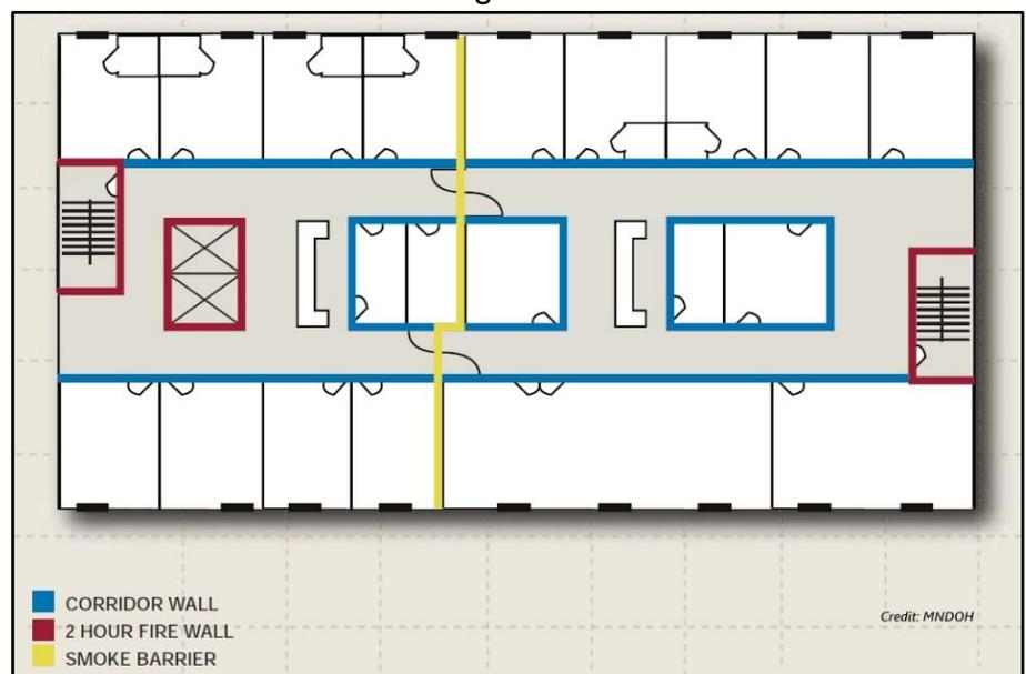
In the second example, a designated smoke zone is used to temporarily create an infectious disease isolation zone. Smoke zones are designed with smoke barriers and fire-rated doors to prevent smoke from migrating to other zones. This property can be utilized to isolate infectious patients. In addition, the area can potentially be placed under negative pressure by using a HEPA-filtered negative air machine to discharge filtered air to the exterior or to the return (exhaust) air system.
