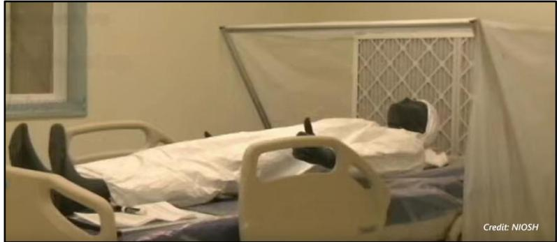
The NIOSH prototype ventilated headboard is a DIY (do-it-yourself) portable, retractable,
